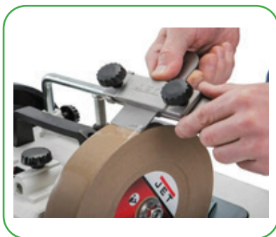
15-rasm. Charxlash stanogida charxlash
