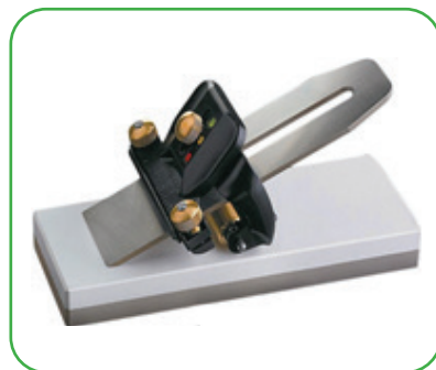
17-rasm. Tig'ning qirovini to'kish
