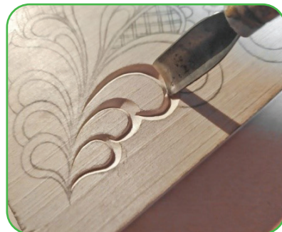
31-rasm. Yog'och o'ymakorligi jarayoni
