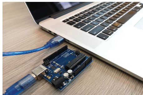
4-rasm. Dasturni Arduino UNO platasiga yozish
