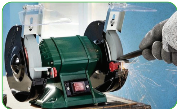
55-rasm. Zubiloni charxlash jarayoni
