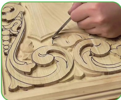
31-rasm. Yog'och o'ymakorligi jarayoni
