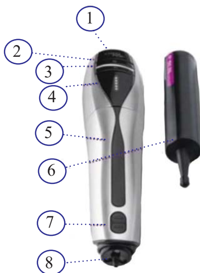
106-rasm. Sovuq 3D ruchka tuzilishi: 1 – quvvat manbayi; 2 – yoqish va o'chirish tugmasi; 3 – LED ekran, 4 – tezlik darajalari; 5 – batareya; 6 – suyuq polimerli kartrij kapsulasi; 7 – ishlash rejimini boshqarish tugmasi; 8 – LED yoritkichlar.
