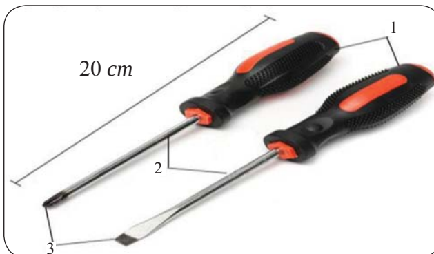
63-rasm. Otvyortka: 1 – dasta; 2 – sterjen; 3 – ishchi qism (uchi).
