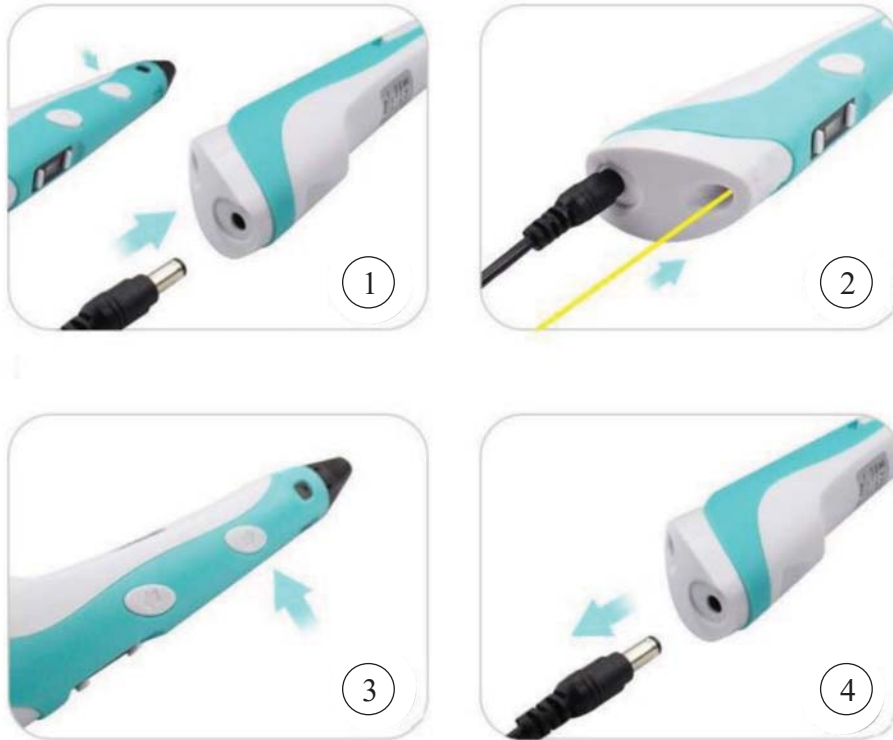
104-rasm. Foydalanish tartibi: 1 – quvvat manbayini ulash; 2 – plastik simni vertikal ravishda joylashtirish; 3 – kerakli haroratni rostlab, oldinga o‘tkazish tugmasini bosish; 4 – ishni tugatgach, quvvat manbayini elektr tarmoqdan va 3D ruchkadan uzish hamda plastik simni chiqarish.
